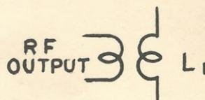
Inductive coupling by means of a hairpin loop or one turn coil coupled to either inductance will result in a greater power transfer to the driven circuit, such as, antenna or a power amplifier, Fig. 3. A single pole, double throw switch may be arranged to change the grid leak to a high value so that superregeneration will result, allowing the use of the oscillator as a trans-
