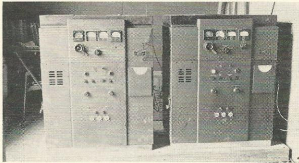
LEFT: After moving to permanent buildings the GI broadcasters installed these two BC-610 E transmitters, modified slightly for continuous service broadcasting.
