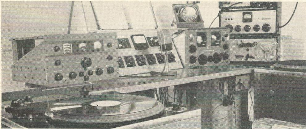
This was one of the later arrangements at "Kilroy," after moving from the temporary vans to quonset buildings. Here are two RCA 70D turntables, and RCA 91A radio, Gates 52 CS consolette, Hammarlund SP 600 radio, and a Magnecord PT6-P tape recorder.
