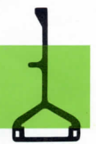
155767 Slide — Used for operating shift fork by one to six, adjacent function levers
